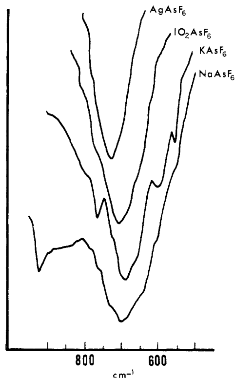
Figure 2.—Infrared absorption spectra of iodyl hexafluoroarsenate compared to silver, potassium, and sodium hexafluoroarsenate.
